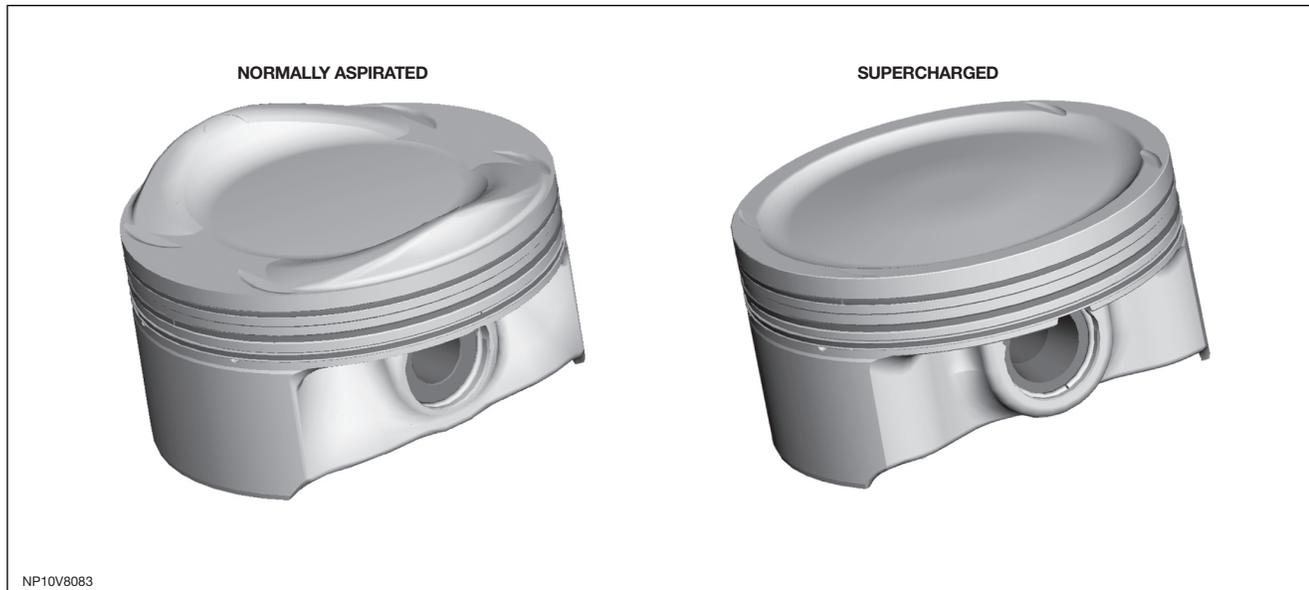
Only one piston grade is available. In a vertical plane, the pistons have a slight barrel form; this is designed to help assure a reliable oil film between piston and block. A solid film lubricant coating is applied to both reaction faces of the piston to help reduce wear and improve fuel economy.
