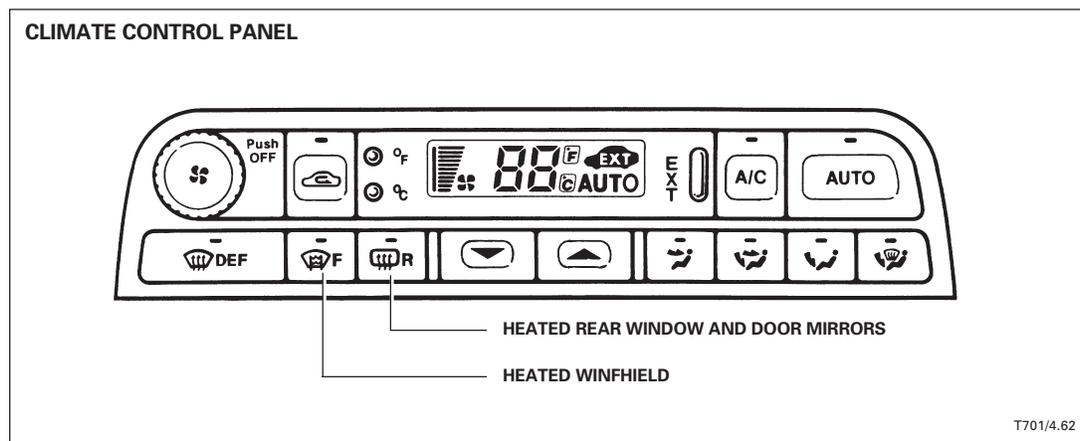
The heated rear window and door mirrors are activated by pressing the “R” button on the climate control panel. The heated windshield can be activated manually by pressing the panel “F” button.
