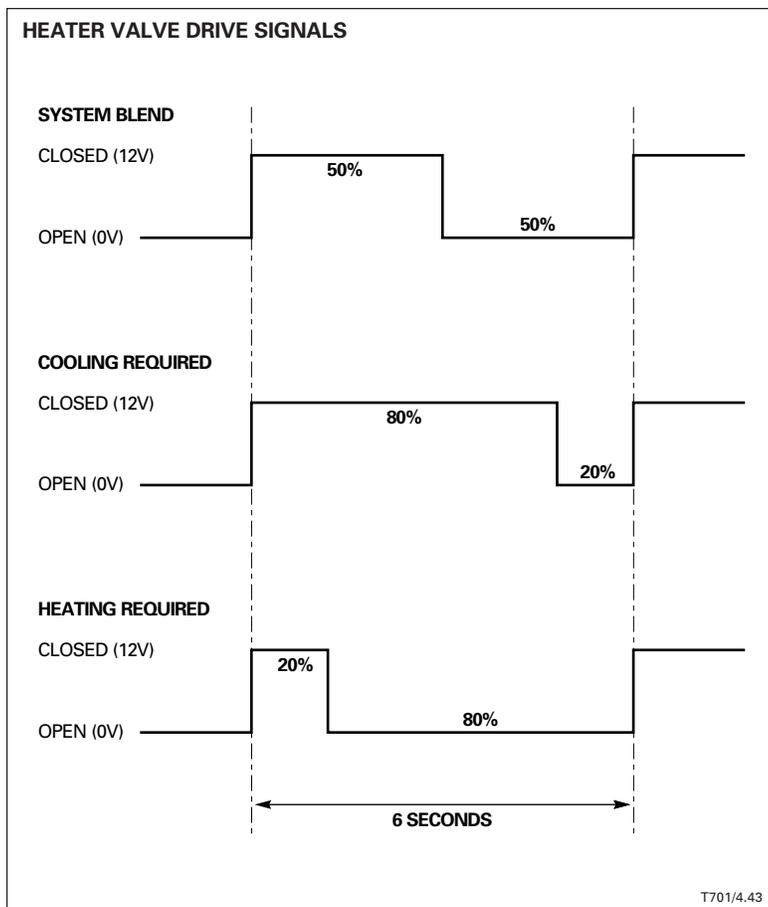
The A/CCM drives the valve with a 12 volt, six second duty cycle signal. The A/CCM increases or decreases the length of the 12 volt signal within the duty cycle to achieve the required heater matrix temperature. If the drive circuit fails (open circuit), the valve defaults to the open position to allow full engine coolant flow to the heater matrix.
