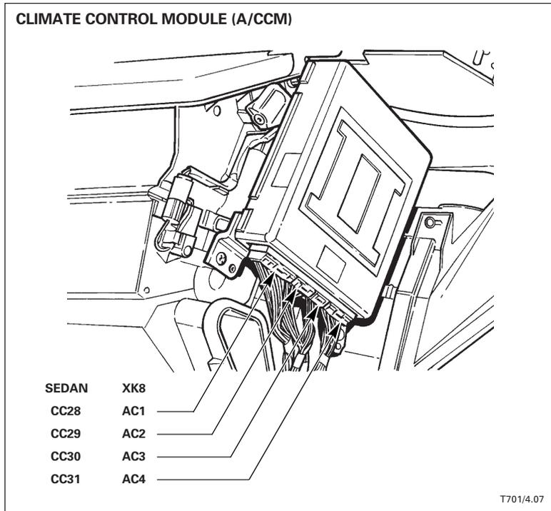
The A/CCM has two microprocessors: one 8-bit and one 4-bit. The 8-bit microprocessor controls the overall system strategy and stores input / output information. The 4-bit microprocessor "conditions" the system signals and processes information.
