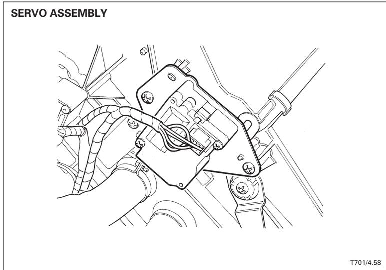
Six air flow control flap servo assemblies are used in the system:
