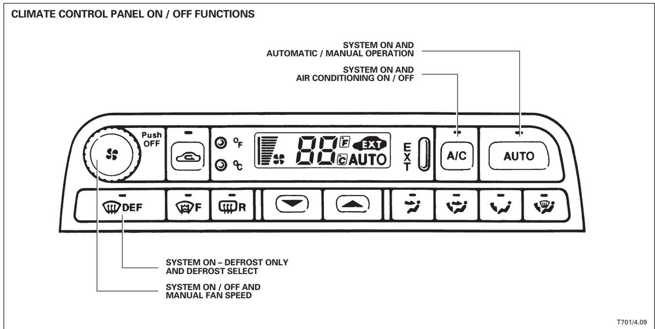
The climate control panel is switched ON by pressing one of the following panel controls:
