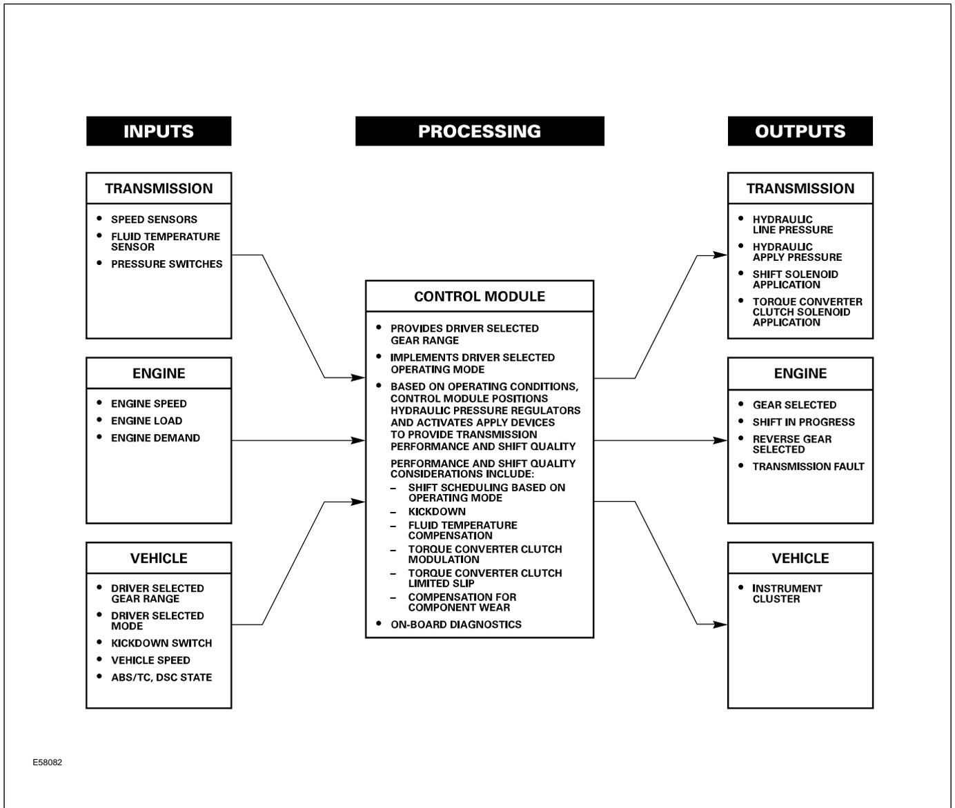
The control module processes the transmission input signals and inputs (signals / data messages) from other systems to perform the following control functions:
