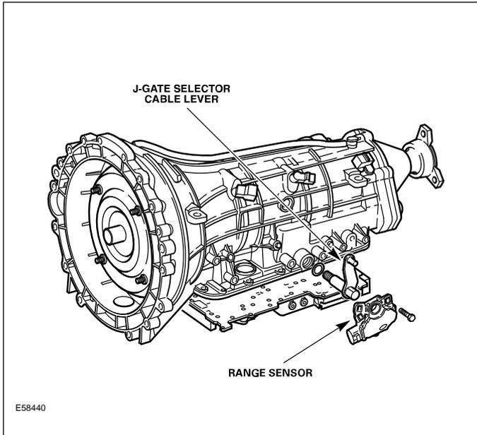
**NOTE:** If the selector cable is incorrectly adjusted, the range sensor may transmit an invalid code, which would cause a DTC to be flagged. Refer to the Jaguar Powertrain DTC Summaries – P0705.
