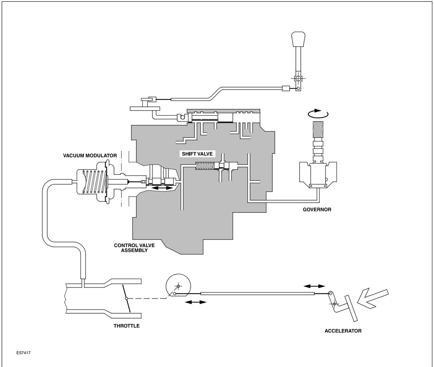
**Electromechanical Control of Hydraulic Pressure**
