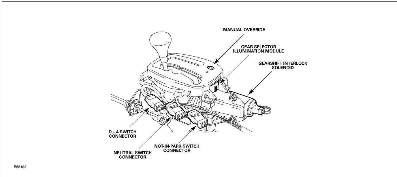
The J-gate assembly incorporates three micro switches:
