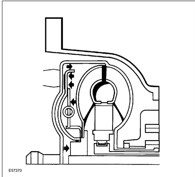
**Lockup Clutch Operation: Clutch Engaged**
