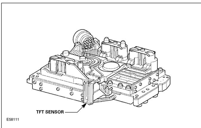
**NOTE:** The TFT sensor is in a series circuit incorporating a Park and Neutral reed switch. The switch is not used for transmission control, and monitoring of transmission fluid temperature is limited to when D or R is selected only. If the selector is in P or N, engine coolant temperature is substituted.
