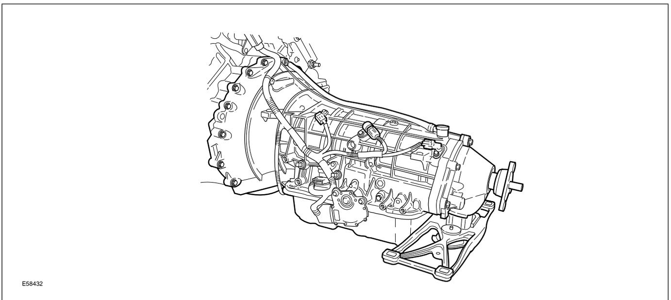
The transmission is electronically controlled by the Powertrain Control Module (PCM), which integrates Engine Management System control. The combined system is known as Powertrain Electronic Control (PTEC). The single control module for both engine and transmission eliminates the need for a high-speed Controller Area Network (CAN).
