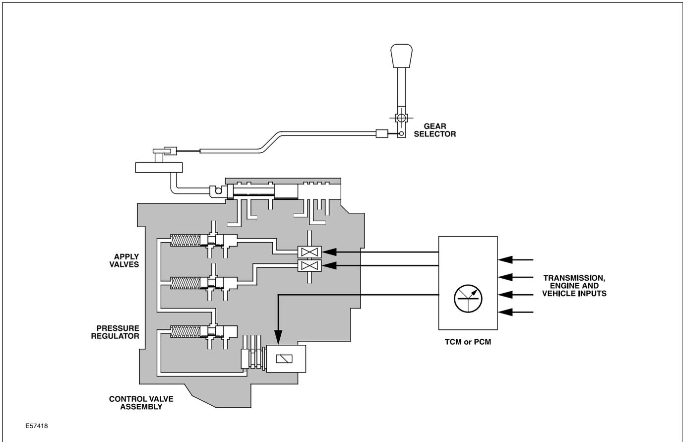
**Gear Selector Position Input to the TCM / PCM**
