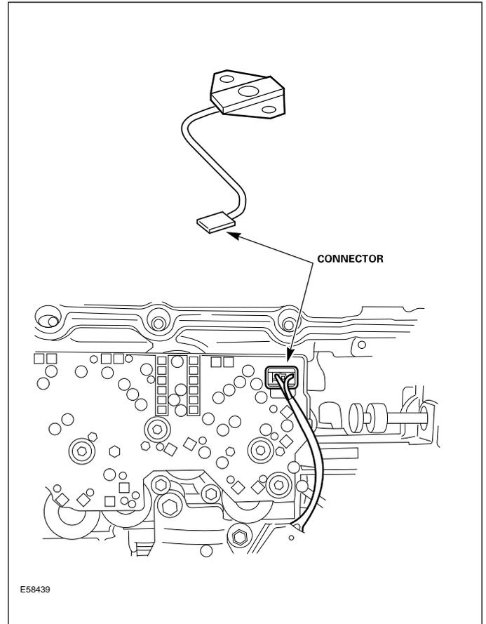
The pressure switch acts a safety switch to prevent simultaneous application of apply elements. For example, if a valve in the valve body gets stuck, it is possible that two elements could apply together causing transmission damage. The switch signals this fault to the PCM, which takes action to prevent the lock up from occurring.
