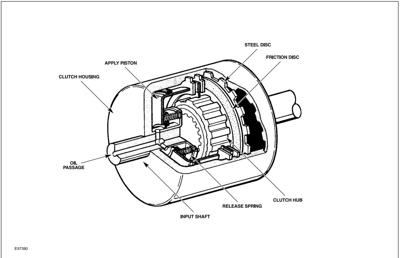
Pressurized oil acts on the apply piston moving the piston in contact with the clutch pack. The hydraulic pressure forces the discs together and the resulting friction connects the discs causing the housing and hub to rotate (or hold) together as one unit. When the hydraulic pressure is released, the clutch return springs move the apply piston away from the clutch discs, allowing them to once again rotate freely.
