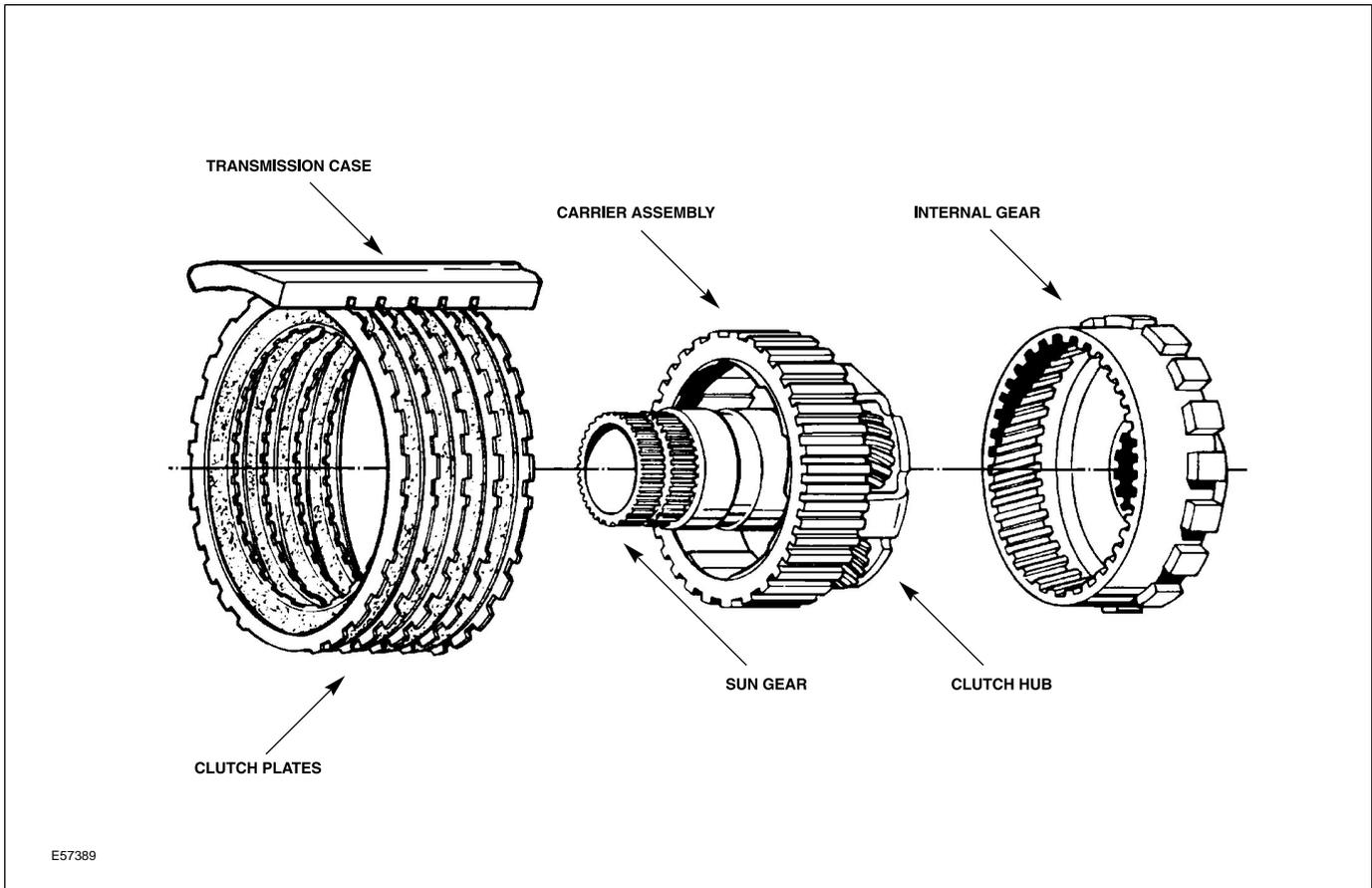
Applying Multiple-Disc Clutches
