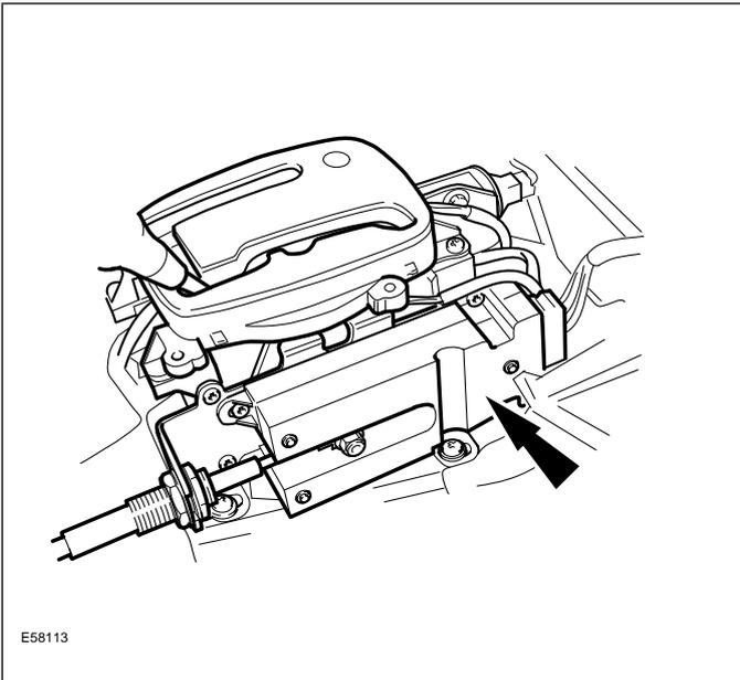
WDS Datalogger readings for the dual linear switch will show as follows: 0 = Closed / low voltage 1 = Open / high voltage
