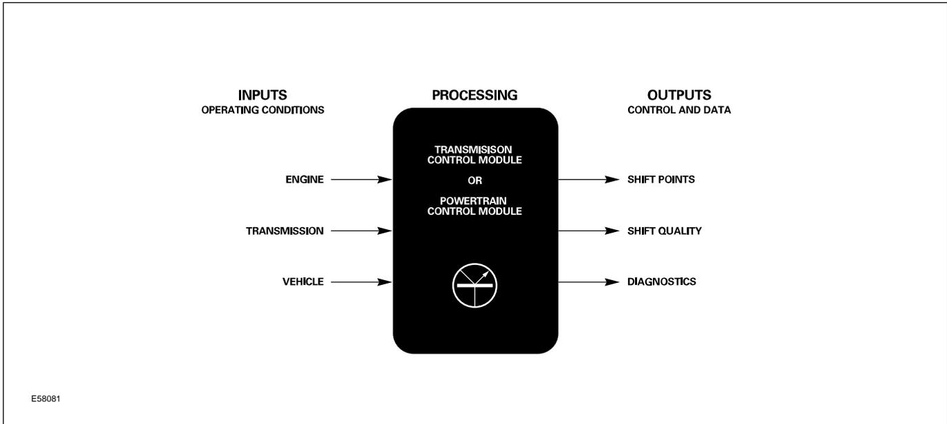
The transmission control module communicates with other vehicle systems, including:
