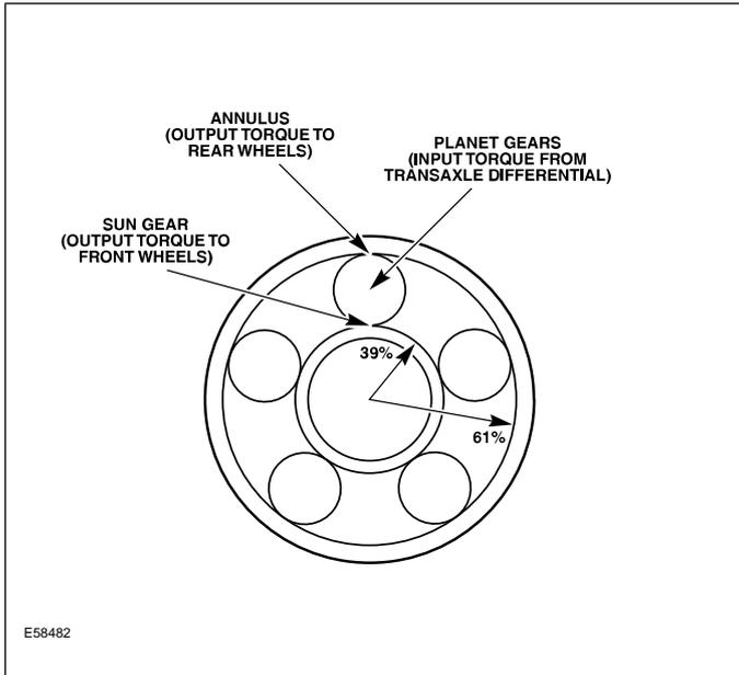
Under normal driving conditions, all the components of the center differential rotate at the same speed, with front and rear torque split determined by the lever ratio of the tooth contacts.
