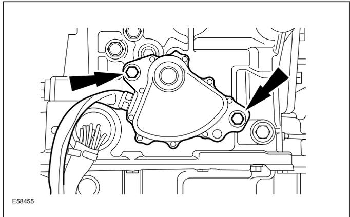
1. Fit the rotary switch to the transmission and loosely fit the 2 bolts.
