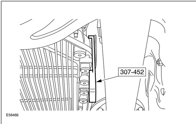
1. Loosen the oil fill plug immediately after starting the engine using special tool 307-452
