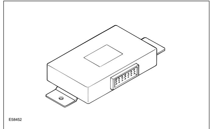
Actual transmission control changes are made by actuators (solenoids) that respond to driver outputs provided by the TCM. These solenoids operate in response to electrical signals; they regulate the control valve operation. The control valves cause changes in the fluid flow passages. These changes result in pressure changes within the transmission.
