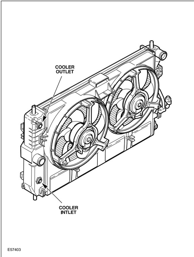
**Separate Oil Cooler (Air to Liquid)**
