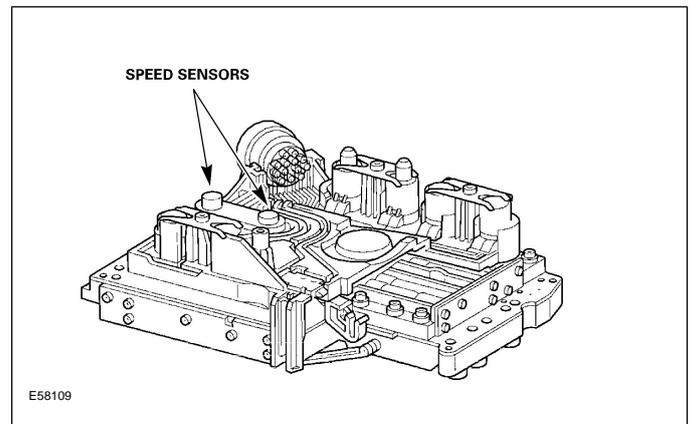
The pickup (coil) portion of the sensors share a common molded platform and mount to the valve body electrical module. The reluctors are impulse rings that are attached to transmission rotating components. To ensure that the correct distance is maintained between the pickups and the impulse rings, the sensors are held in position by a leaf spring that rests against the valve body. The speed sensors are serviceable only as a unit.
