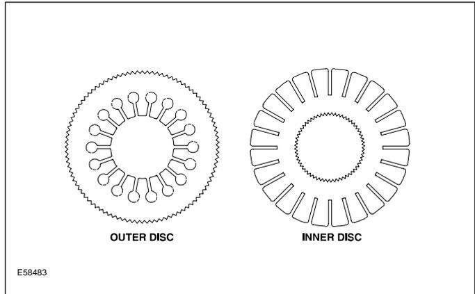
The sun shaft has male splines that connect to the viscous coupling inner hub; the outer viscous coupling is driven by the annulus via four drive pegs. The viscous action only occurs when there is a relative speed difference at the front and rear drive wheels due to reduced traction on either axle.
