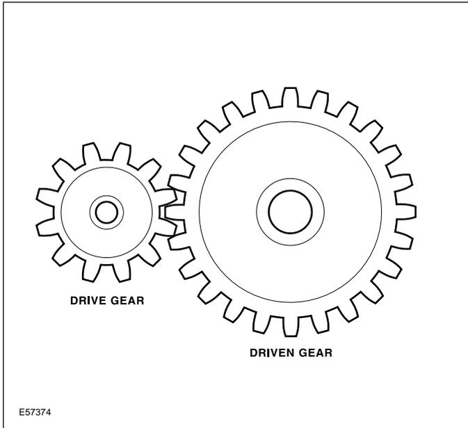
Torque is multiplied or reduced in the opposite of the gear ratio. In this example, the torque ratio is 1:2. The driven gear will turn at half the drive gear speed, however, the driven gear will have twice the torque of the drive gear. Torque is multiplied by two.
