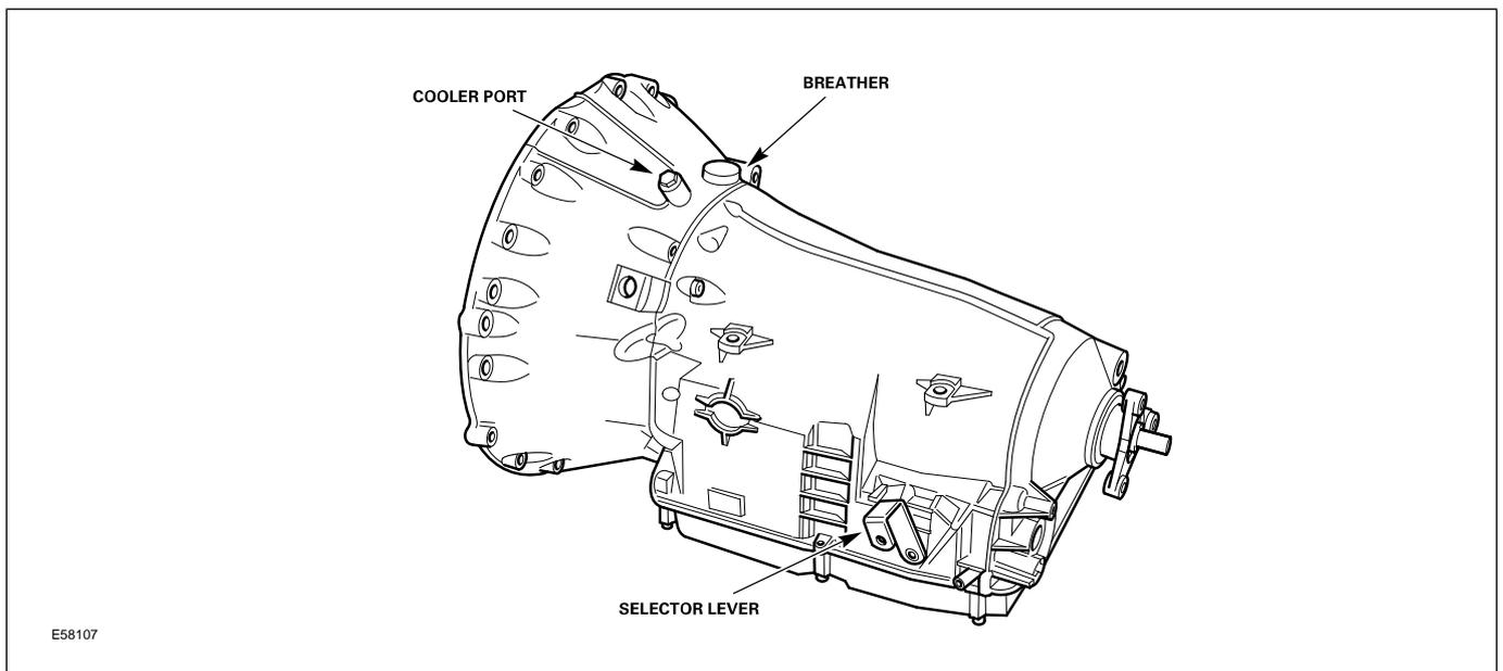
The transmission is TCM (transmission control module) controlled. The TCM communicates with the engine management system, ABS/TC system and the instrument cluster via the high speed Controller Area Network (CAN).
