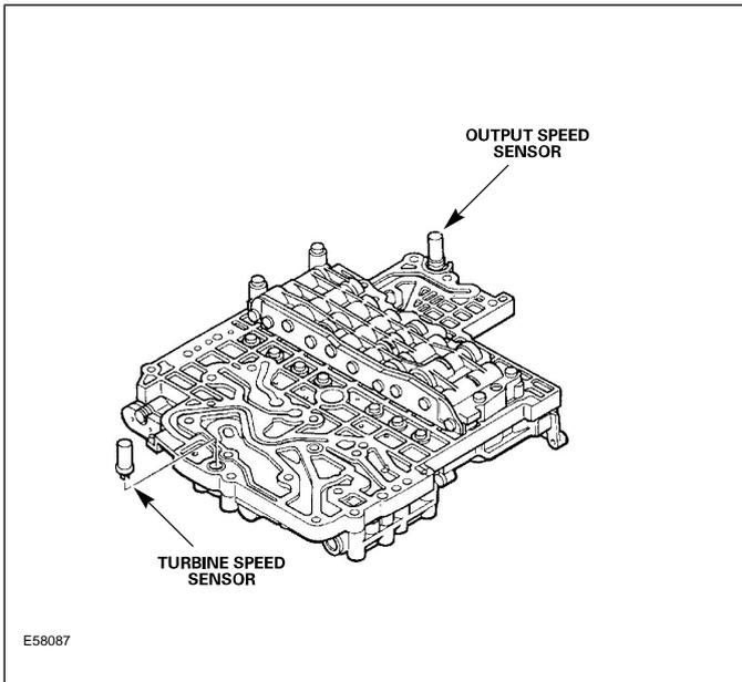
Both speed sensors are inductive pulse generators, which provide the TCM with a transmission speed alternating voltage signal. The pickup (coil) portion of the sensors are mounted to the valve body; the reluctors are integrated with transmission rotating components. The TSS sensor retractor has 30 teeth; the OSS sensor retractor has 36 teeth.
