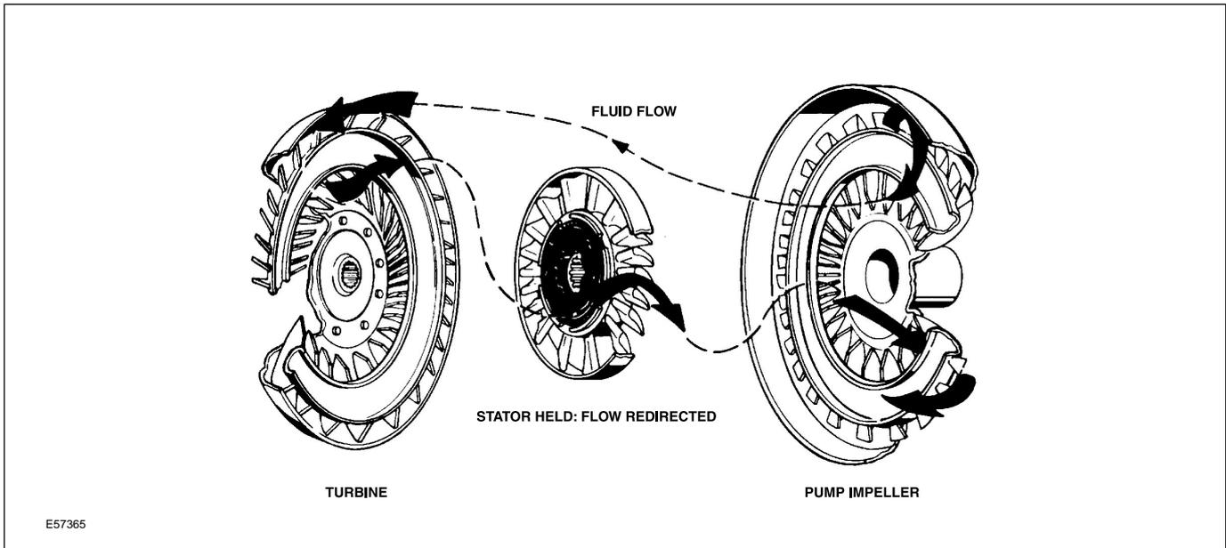
the turbine. The speed of the stator is about the same as the other components. If the accelerator is applied to the point where the pump impeller speed is significantly greater than the turbine speed, the stator clutch will hold to increase torque.
