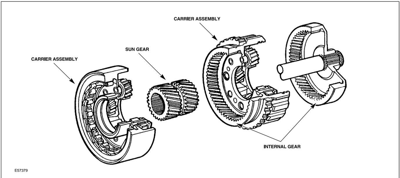
Uses for Planetary Gear Sets
