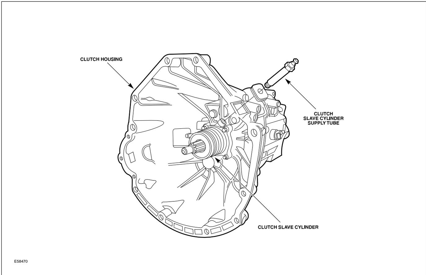
The central slave cylinder is fixed to the clutch housing with four bolts, together with an integrated release bearing press-fit on the clutch slave cylinder.
