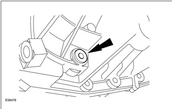
When the transmission is filled, the fluid should come up to the lower edge of the check bore. If fluid is required, fill the transaxle to 0.5 mm (0.02 in) below the lower edge of the fill plug bore.
