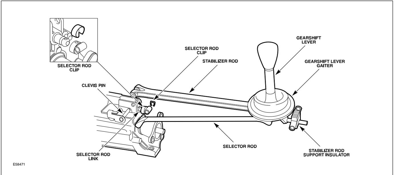
In order to isolate the outer gearshift mechanism from the bodywork, the gearshift housing is located in a remote gearshift mounting that is rigidly joined to the transmission by the gearshift stabilizer. This mounting can move lengthways to balance the rotational movements of the engine/transmission.
