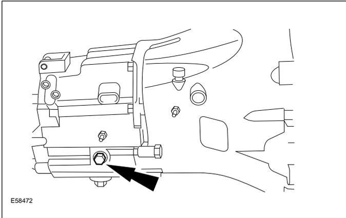
Fill the transmission to 0.5 mm (0.02 in) below the lower edge of the fill plug bore.
