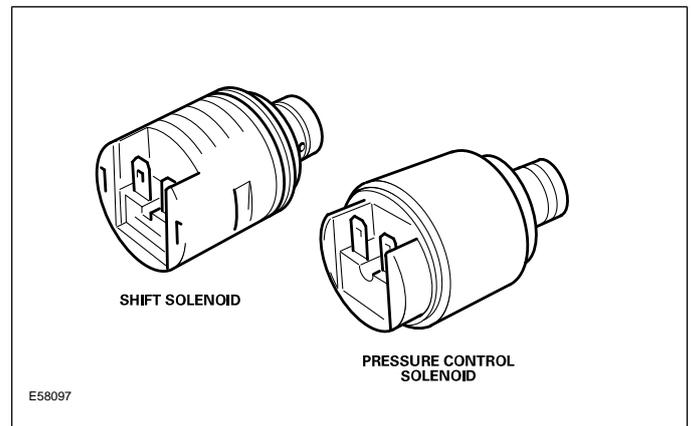
Shift solenoids SSM1, 2 and 3 are used to shift the transmission through all forward gears and reverse. They are two-way on / off normally closed solenoids. The TCM controls the solenoids by switching the ground side of the circuit.
