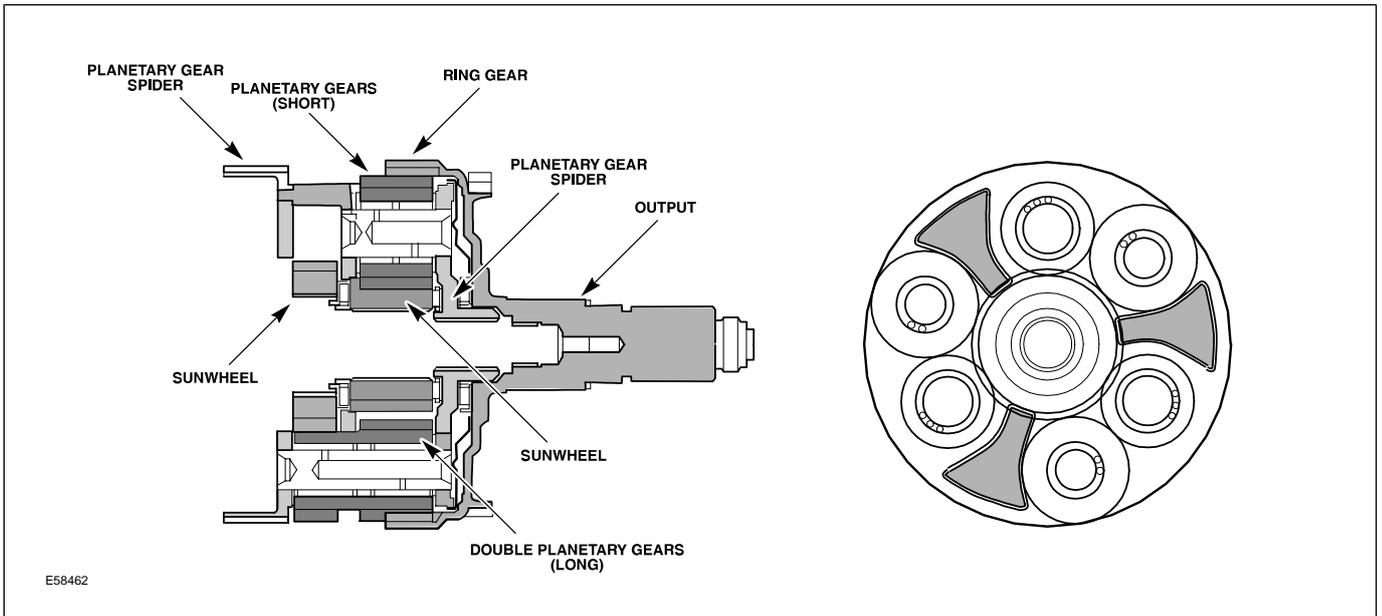
All gear shifts 1st to 6th or from 6th to 1st are power-on overlapping shifts. During the shift, one of the clutches must continue to transmit the drive at lower than main pressure until the other clutch is able to accept the input torque.
