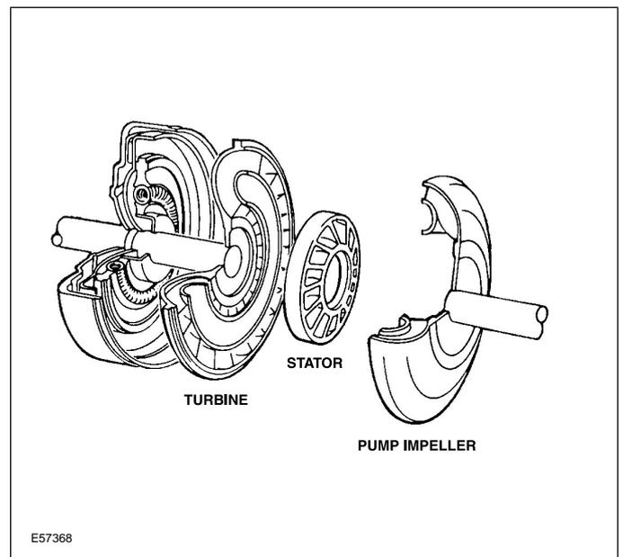
The two plate clutch operates opposite in that it is engaged by hydraulic force directed from the valve body and released by the force of the fluid acting on the pump impeller. The clutch connects the converter housing and the pump impeller assembly.
