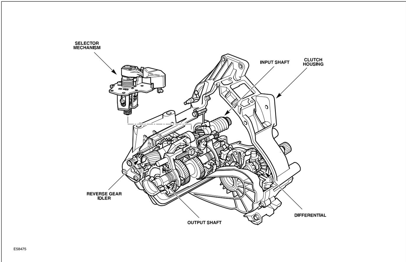
To further improve stability and gear shifting, a maintenance-free cable operating mechanism is used. All the gear wheels, including reverse gear, are helical cut, synchronized, and run on needle roller bearings. First, second, and third gear have double synchronization. The advantages of double synchronization are that the transmission runs quietly, gearshifts are smooth, and the assembly is compact and light in weight.
