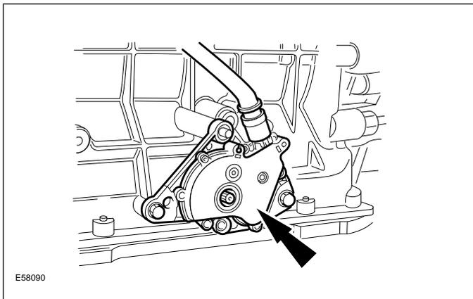
**NOTE:** If the selector cable is incorrectly adjusted, the range selector may transmit an invalid code, which would cause a DTC to be flagged.
