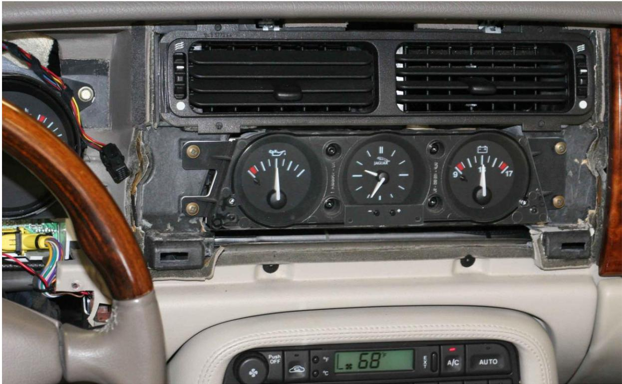
23. Reconnect the battery. The normal indications are in the photo above. The red fault lights on the voltmeter and oil pressure gauges should also briefly light up as part of the test sequence just after starting the car. Also check that the gauge illumination is working properly. You will also need to reset your windows after reconnecting the battery.
