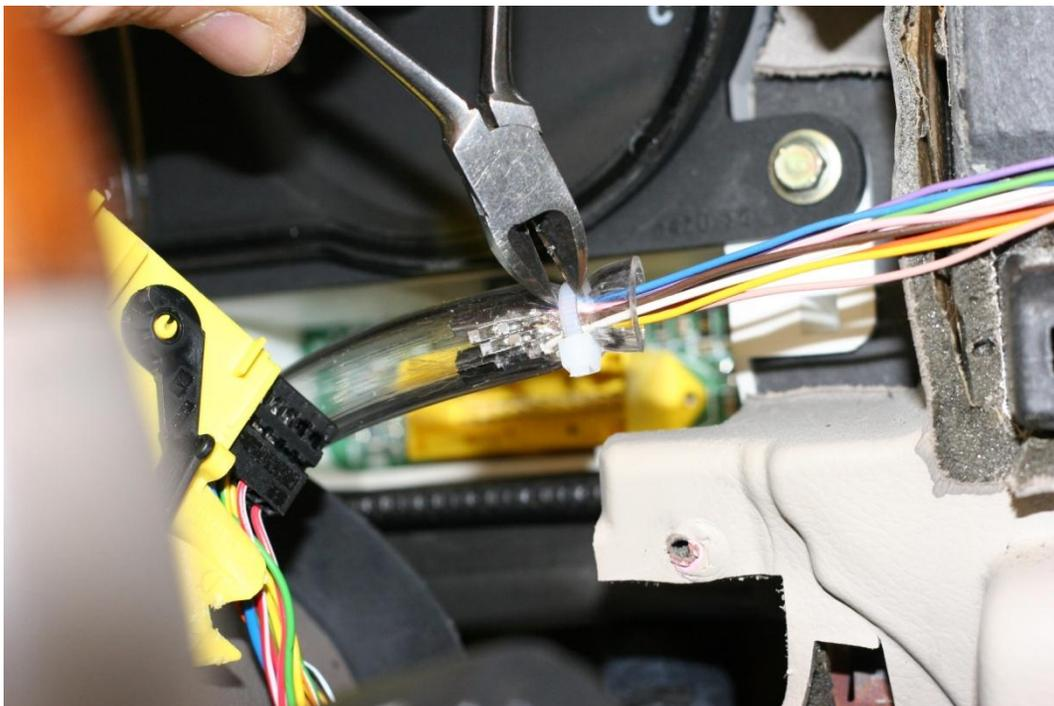
9. Note that there are two navigation connectors. One is 12 pins and the other is 16 pins. Locate the 12-pin connector and attach the Posi-tap connector tap to the PINK and BLACK wire. Follow the Posi-tap instructions: <http://www.posi-lock.com/instructions1.html>.
