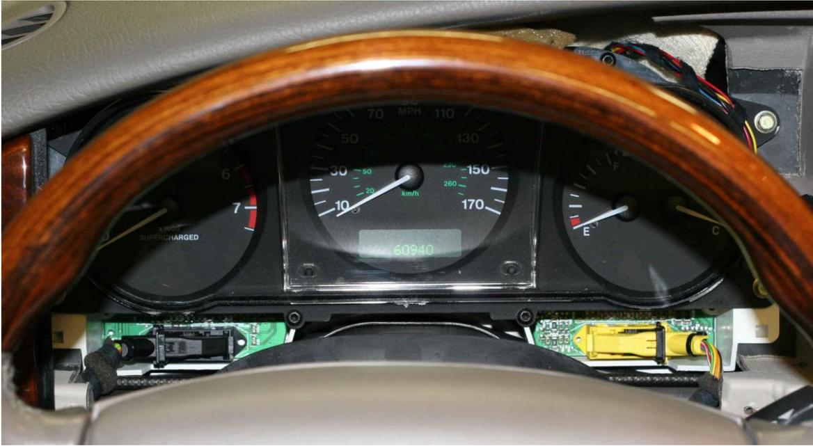
12. Release each of the connectors by depressing the tab-lock (pointed to in photo below) and pulling the hinged black plastic bail away from the wire end of the connector.
