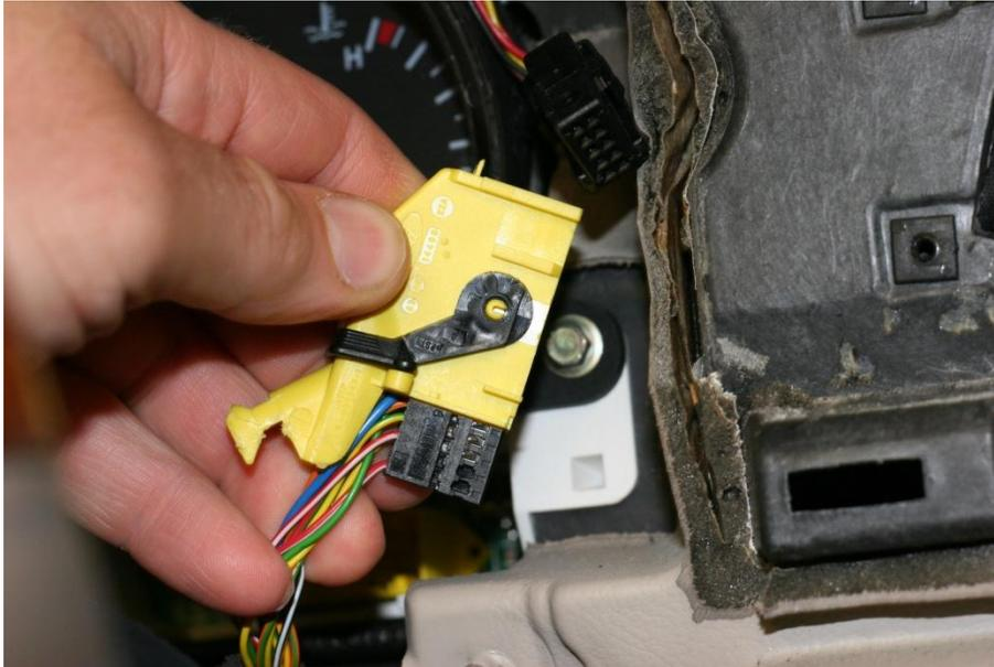
16. Insert the terminals in the connector bodies. Note that the pin number for each corner pin (1, 13, 14, 26) is embossed in the connector body. The tab on the connector pins must face the window in the connector body.
