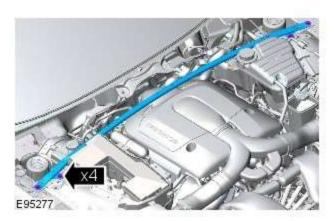
2. Remove the engine compartment brace.
