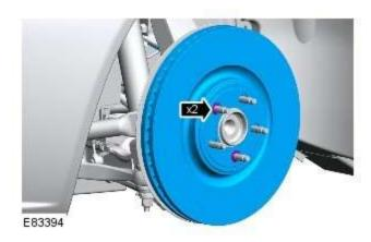
5. Remove the rear brake disc.
