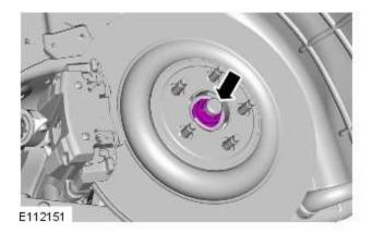
15. CAUTION: Do not use air tools to install the nut. Failure to follow this instruction may result in damage to the component.
