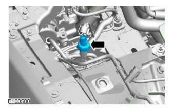
4. CAUTION: Make sure the air conditioning (A/C) hose does not turn when removing the low pressure switch.
