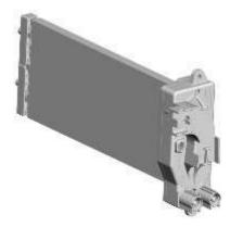
The electric booster heater is installed in the heater assembly, on the downstream side of the heater core. It consists of ceramic coated thermistor elements, rated at 1.25 kW, and a micro-controller. Electrical power for the booster heater is supplied by the  $\underline{BJB}$  via a 150 A megafuse installed under the  $\underline{RH}$  front seat.
