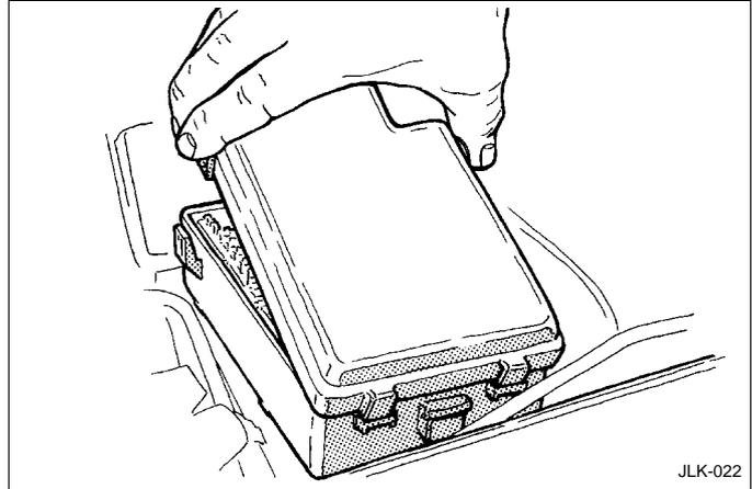
A second fuse box is situated within the bulkhead extension on the passenger's side.
