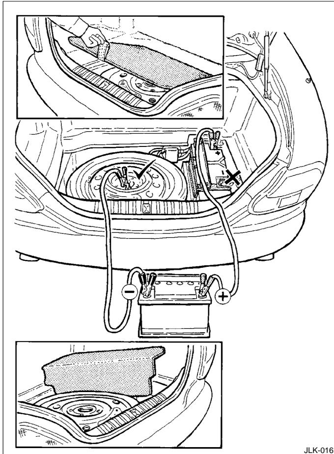
**Caution:** Do not connect the negative jump lead directly to the negative (-) terminal of the discharged vehicle.
