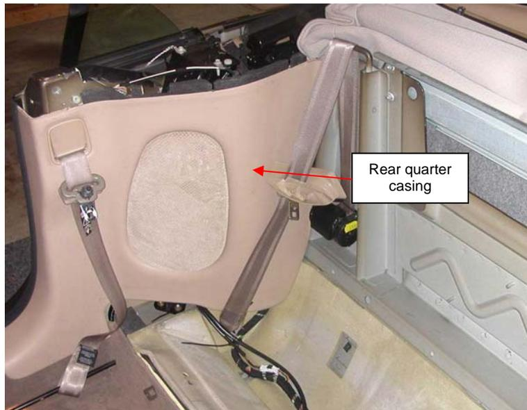
Fig. 7 Rear seat area with squab removed
