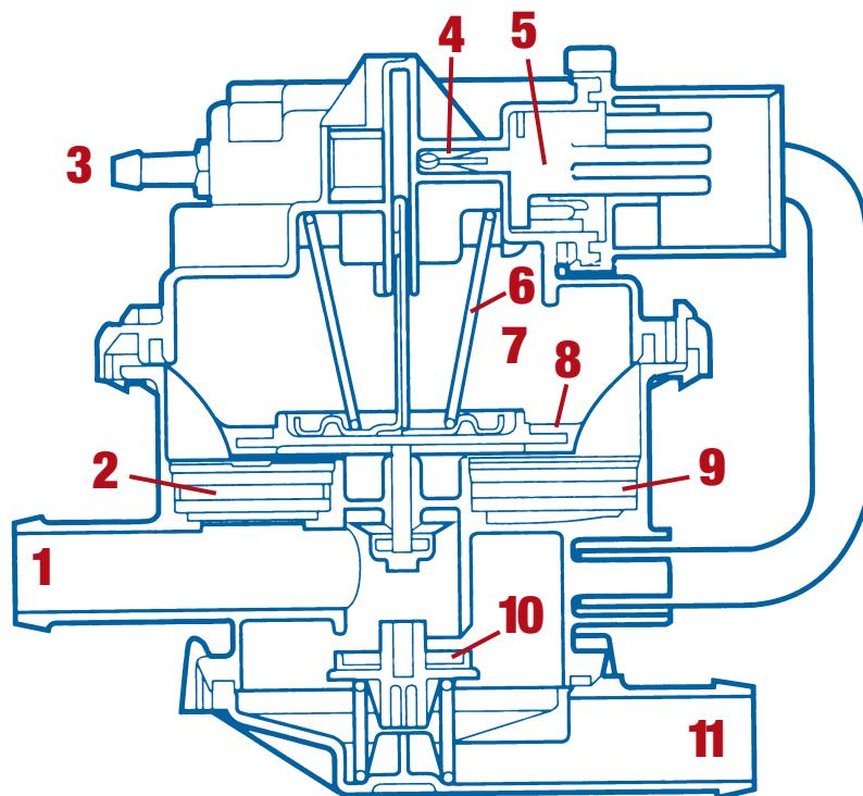
**The key to Chrysler's LDP is the reed switch. When the diaphragm is all the way down, the vent valve is pushed open.**
