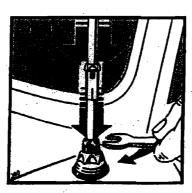
Tighten threaded bushing, then extend and retract telescope again to check function.
