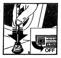
Switch radio off and drop the plastic wire into the mounting hole until teeth are engaged by the drive. If the plastic wire is not pulled into the drive, the drive has not engaged the teeth. If this occurs, switch radio off and on and turn plastic wire up to 180 degrees until teeth on wire connect with the drive. As the plastic wire is drawn in, gently push the telescope's tubes into the housing. Then insert the threaded bushing.
