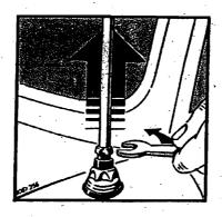
Extend telescope as far as possible by switching the radio on. Loosen threaded bushing until it is free from the antenna head. Remove the telescope with its plastic wire by pulling the telescope upward. Note the direction in which the teeth face.
