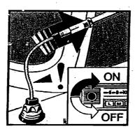
Switch radio off for a moment and then on. This should fully extend the telescope and toothed plastic wire. Do not extend the telescope by hand. The electronic control limits duration of operation at approximately 12 seconds.
