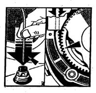
Insert plastic wire through mounting hole until it comes to a stop. Be sure to arrange wire with teeth facing in the same direction as the removed telescope.
