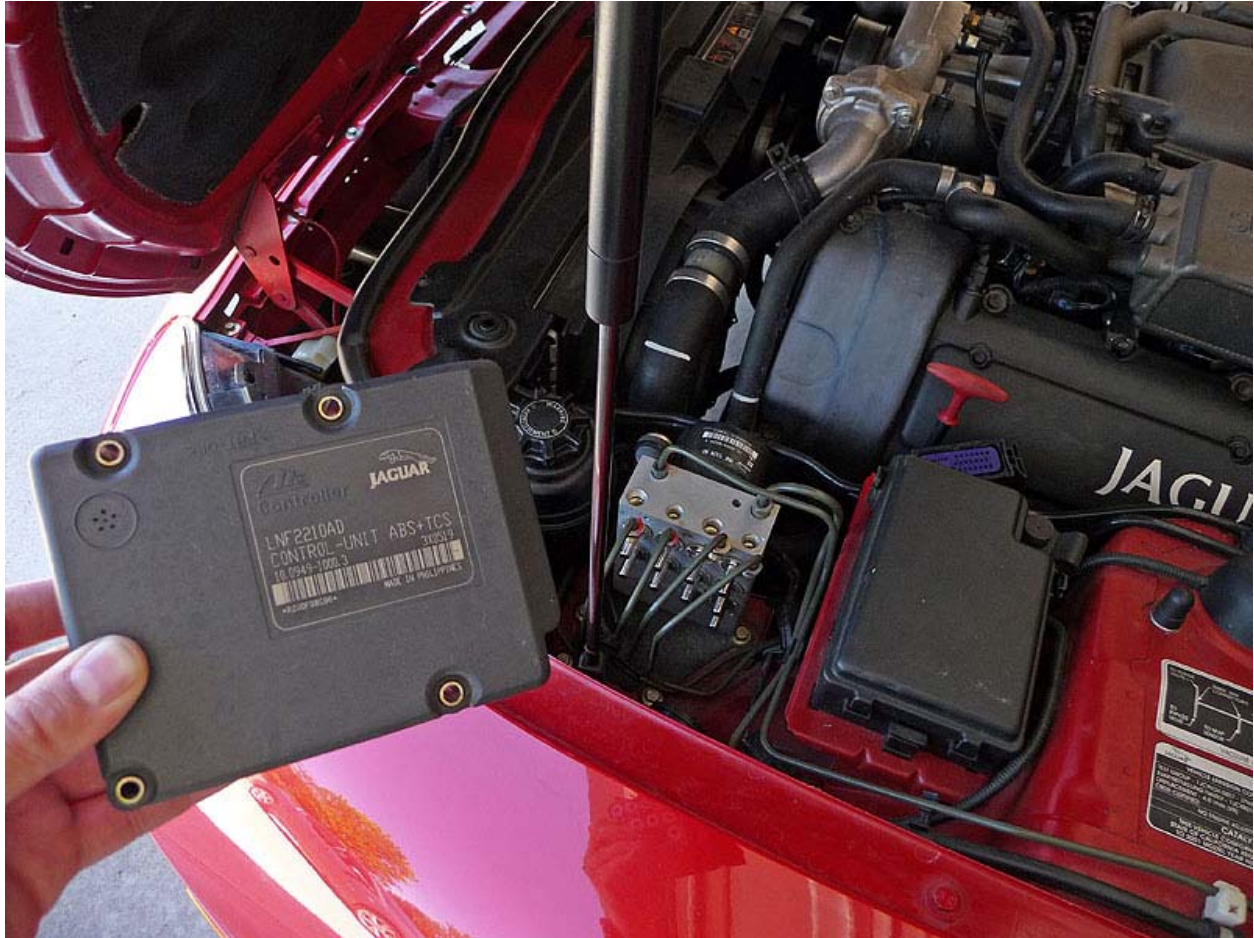
Control Unit Opened
