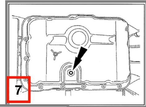
**8: Install the fluid level and fill plug adapter into the fluid drain plug**
