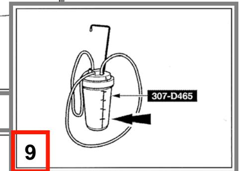
**10: Hang the fluid transporter/evacuator/injector under the vehicle. Position it upright and close to the transmission**
